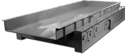
*Brute Force Feeders* – are single mass Mechanical Feeders powered by twin rotary motors. They are a very simple design and handle shock loading well, but lose power under heavy head loading. These units are very easy to repair, because you simply change the weighted motor.
