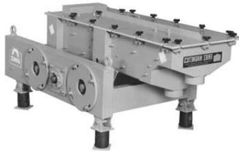
*Horizontal Motion Conveyors* – The E-Z Slide™ Horizontal Motion Conveyor is ideal where gentle handling of self-cleaning is required such as in snack foods or processing of friable products. The unique drive causes the tray to move forward slowly carrying the product, then reverse rapidly, causing the tray to slide back quickly.
