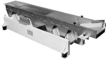
*HV Conveyors* – is a heavy duty two-mass Mechanical Conveyor designed for coal, glass, and aggregate type applications. It can be supplied with replaceable AR liners. It uses a unique rubber spring that can be adjusted for the optimum drive angle.
