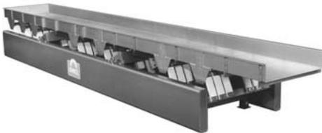
*SM Conveyors* - Single mass units are Eriez' least expensive mechanical conveyors, because they use the floor or base as their reaction mass. This allows for a low profile and efficient system to convey materials and parts. These efficient single mass conveyors move light loads of bulk materials at flow rates up to 18 tph (16mtp/h).
