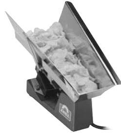
*High Deflection Model Feeders* – These unique Electromagnetic Feeders operate at a higher (4.76 mm) amplitude and lower frequency (30 CPS) enabling them to handle hard-to-feed materials such as fine powders and flexible leafy products. The HD series can handle up to 19.82 cubic meters/hour of light products such as cereal weighing 4.53-6.8 Kg/cubic feet.
