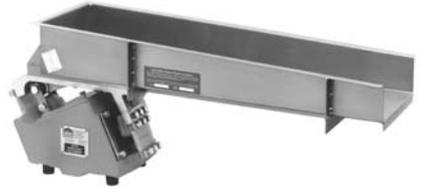
*High Speed Model Feeders* – The HS Feeder is a variation of the A and C models designed mainly for packaging and production applications requiring frequent on/off cycling (up to 100 times/minute). Being designed mainly for food packaging applications, they can operate at up to .090" (2.28 mm) amplitude at 50-60 cycles and feed up to 600 cubic feet (16.9 cubic meters)/hour of materials weighing 30-40 lbs (13.6-18.1Kg)/cubic feet.
